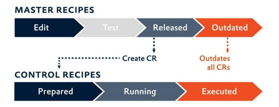
The use of zenon functions allows for external systems such as a MES or ERP system to create, start, and control production Control Recipes from known Master recipes.
