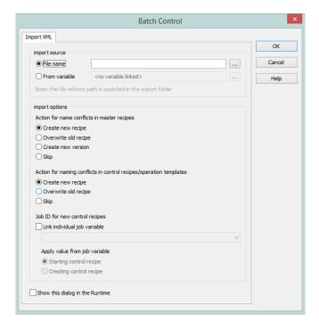
The figure above displays the zenon function call 'Import batch recipes' which will import a recipe into the zenon Runtime system. To import a Master Recipe the source information where the actual Master Recipe is stored, and how to handle conflicts of the same Master Recipe name must be specified.
