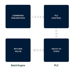
When the phase is active in the batch recipe, the set point value is sent to the PLC, together with the start signal.
