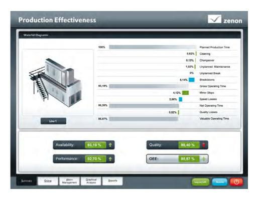
Figure 2: Identifying improvement potential with zenon by standardizing the OEE Waterfall Diagram
