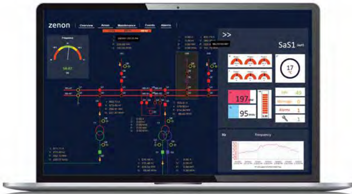
Compact view of the grid configuration in the single-line diagram; additional indicators increase clarity.
