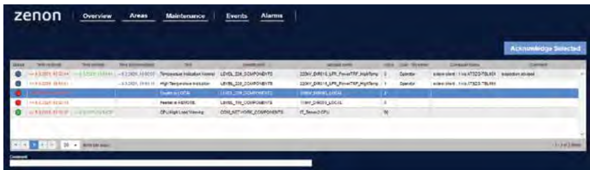
The Alarm Message List and Sequence of Events List (SoE) provide detailed information about all processes and equipment.
