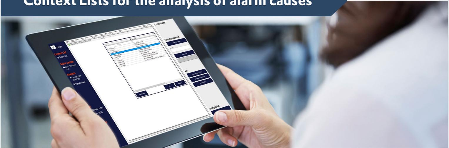
The new “Context List” screen type helps zenon users to structure manually-entered data. Analysis of the alarm causes is one area where it is used. Descriptions of alarm causes are pre-defined and harmonized in the Context List. As a result, it is ensured that each operator uses
