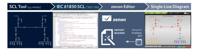
From an SSD file to a single-line diagram
