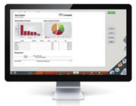
Figure 1: Example of an F&B alarm report in zenon. The bar chart on the left side provides information regarding the alarm duration per machine; the pie chart on the right shows the number of alarms per machine.
