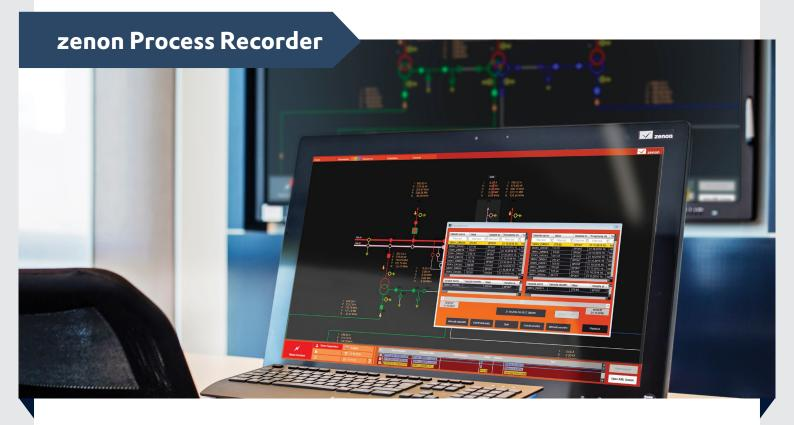
The Process Recorder is a new module that is offered in zenon 7.60. It is used to record processes completely. If existing tools, such as the Alarm Message List or the Chronological Event List, cannot record things with enough traceability, the Process Recorder provides information on the precise processes during operation. Events and status
