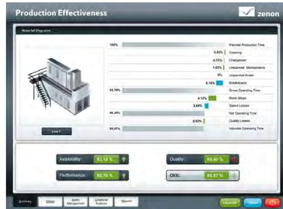
Figure 4: Using zenon, the calculation and display of real time performance indicators is made possible without programming – simply by means of setting parameters.
