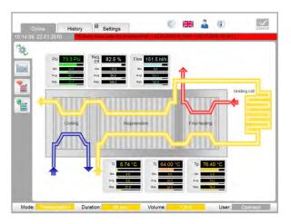
Figure 2: Historical and real time information, easily available thanks to zenon, improves control of the pasteurization process.
