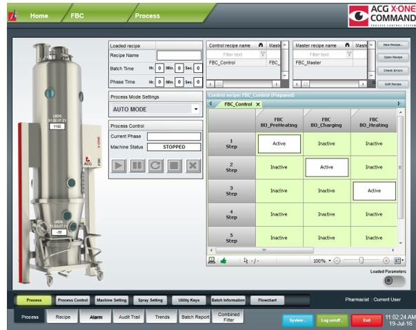
Figure 4: ACG X-ONE COMMAND system: Batch recipe.
