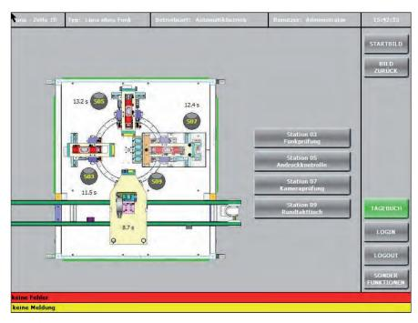
For a better overview, machine and equipment layouts are integrated into the application and the control panels at the individual stations.
