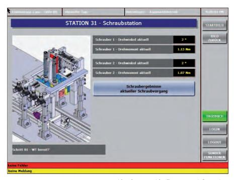
zenon provides the user with all necessary information, such as the angle of rotation or torque, at a glance.
