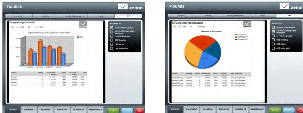
The zenon application shows the down times of the equipment very clearly (left) as well as individual problems with the different robots (right) – once for the whole duration and once for the duration adjusted for breaks.
