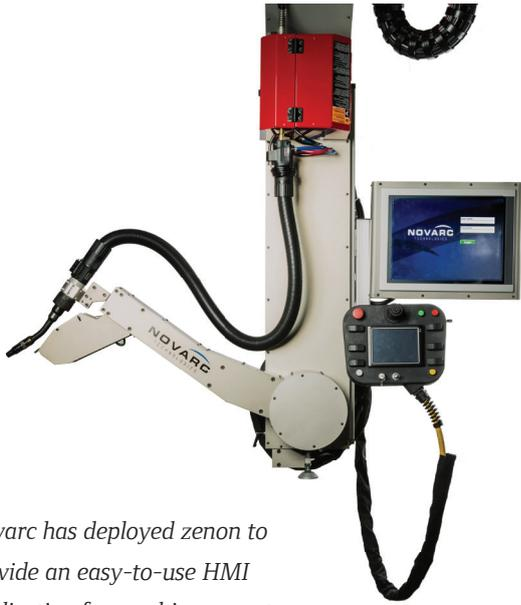
*Novarc has deployed zenon to provide an easy-to-use HMI application for machine operators.*
