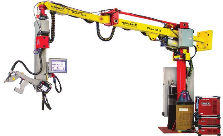
*zenon delivers an intuitive user interface on both the spool welding robot control screen and the companion pendant.*
