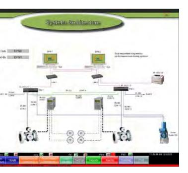
System Architecture, showing zenon in dual-redundant mode.
