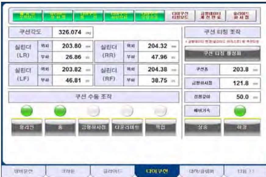
With intuitively designed screens operators gain access to many valuable data such as the press machine status (e.g. cushion angle, location of each cylinder, press machine movements and much more).
