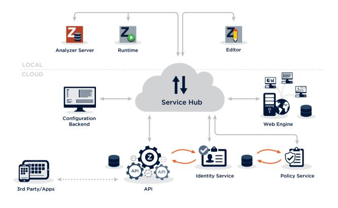
Figure 1: All components in the zenon Service Grid are connected via the central Service Hub. This also constitutes the connection between the local level and the cloud.
