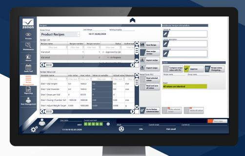
flow management, and recipe management are an integral part of the software platform. Engineering with zenon also provides versioning, change history and documentation to support the validation process. Detailed diagnostic options assist further; for example, to quickly identify problems in communication.
