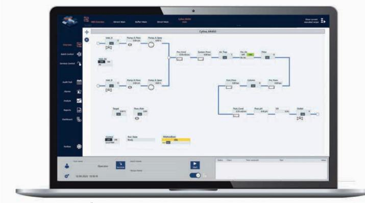
Figure 3: P&ID of the ÄKTA ready™ 450 Chromatography System in the zenon POL.
