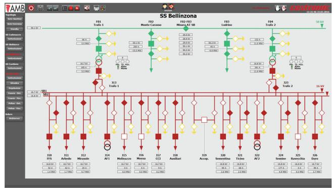
When distributing from 50 kV to 16 kV, the status of each line is shown exactly using ALC.
