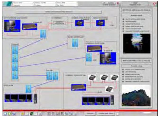
Simplified diagram of the Ethernet supervision system network
