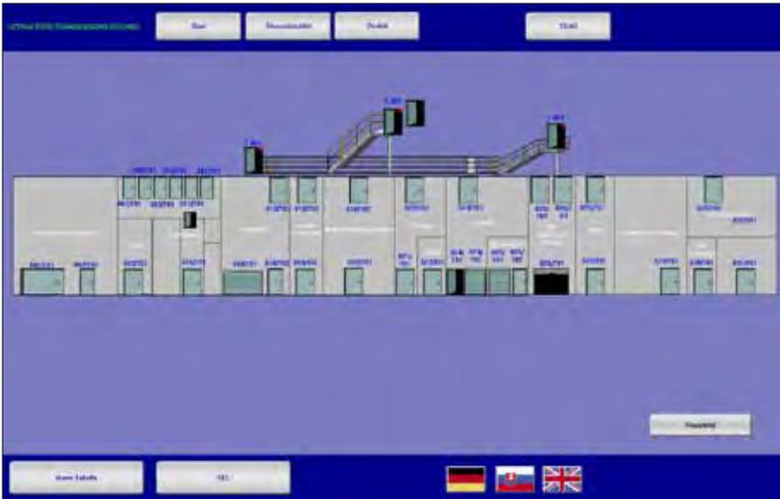
*zenon visualizes and monitors the transformer stations, energy consumption, lighting control, control of blinds and the doors of the production complex.*
