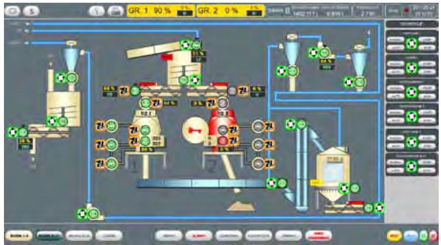
Visualization and control of the rending machine - for shredding of raw material.
