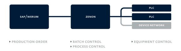
zenon provides the translation from a supply chain production order in the business IT, to control each required process on the OT system. zenon receives the production order through the defined ERP or MES connection, maps these to a Master Recipe, creates a Control Recipe, and when requested starts the production execution. Production status and key values are communicated back up from the equipment to the ERP or MES.
