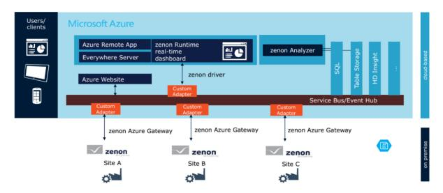
The Azure cloud technology integration into zenon is highly scalable in scope and functionality, effectively extending the zenon structure. For example, historian data can be moved to the cloud enabling efficient data management, storage and analysis; live processes can be communicated opening the possibility of global visibility; with the zenon Analyzer being available as a cloud solution.
