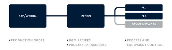
zenon provides the translation from a supply chain production order in the business IT, to orientate and execute specific production processes on the OT system. zenon receives the production order through the defined ERP or MES connection, maps these to a Recipe, communicates the correct parameters to the correct production machines, then issues a start command. Production status and key values are communicated back up from the equipment to the ERP or MES.
