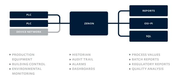
zenon uses its communication library to connect to all production equipment and devices, variables are defined in an alarm structure, and in a historian structure. Using either the Report Viewer or zenon Analyzer, reports can be generated automatically or manually, and stored on a secure server.
