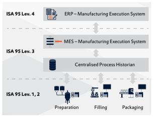
Figure 1: Classic OT - IT integration based on a hierarchical model.
