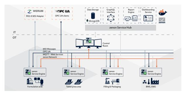
Figure 4: zenon as a modular automation integration layer, including data storage, reporting and IT integration.
