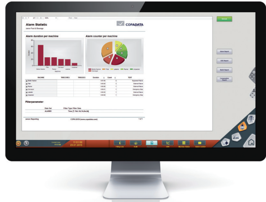
Figure 1: Example of an F&B alarm report in zenon. The bar chart on the left side provides information regarding the alarm duration per machine; the pie chart on the right shows the number of alarms per machine.
