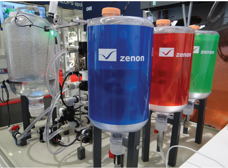
Figure 2: The portable tank model provided real-time values from various sensors to zenon and worked similarly to a real production facility.
