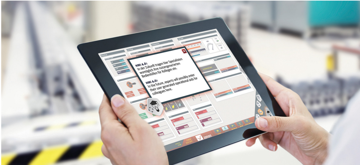
Figure 4: Example of a user-generated operating aid within a zenon HMI application to solve a specific problem.
