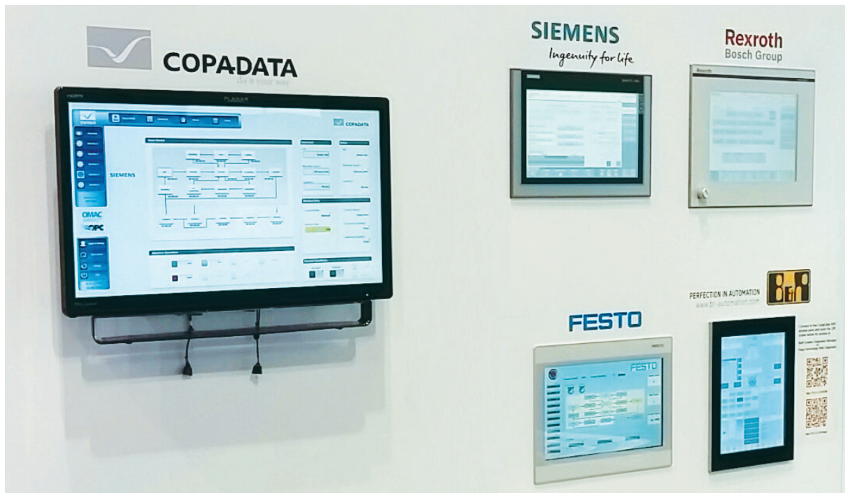
Figure 1: PackExpo exhibition in Chicago, fall 2016: the leading suppliers B&R, Bosch Rexroth, COPA-DATA, Festo and Siemens presented an initial interoperability demonstration based on OMAC PackML and OPC UA standardization.
