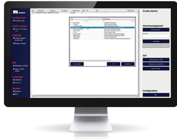
Figure: The context list allows manually-entered data to be arranged. So alarm causes, for example, can be pre-defined and thereby used for later analyses.
