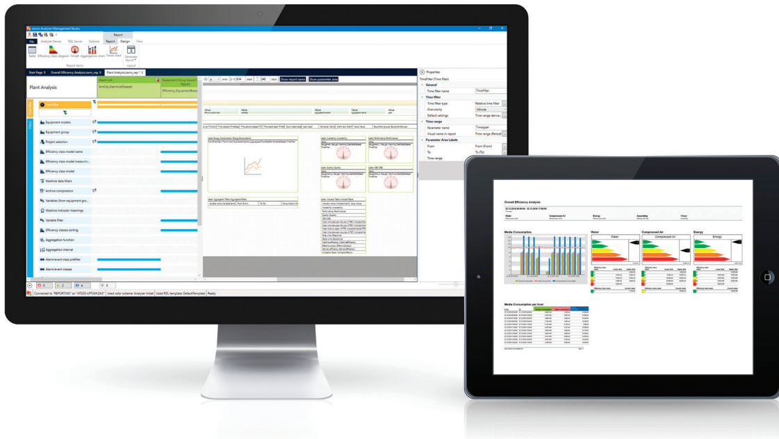
Figure 1: Configuration and design of a report with trend diagram and OEE measurement instruments in the zenon Analyzer Management Studio. Display of a report in bar chart format, several efficiency class diagrams and a table in the Report Launcher.
