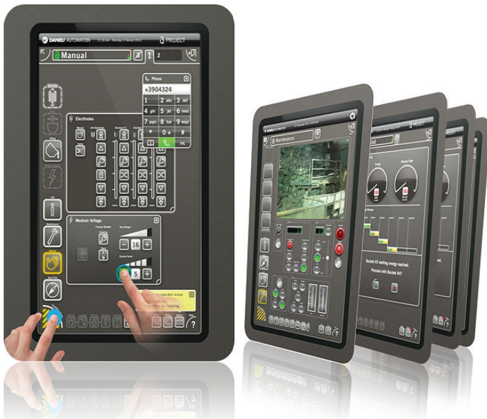
Figure 1: Operator Assistant (OA): The innovative Multi-Touch operating interface by DIGI&MET, part of the HCI extended metal automation platform named 3Q.
