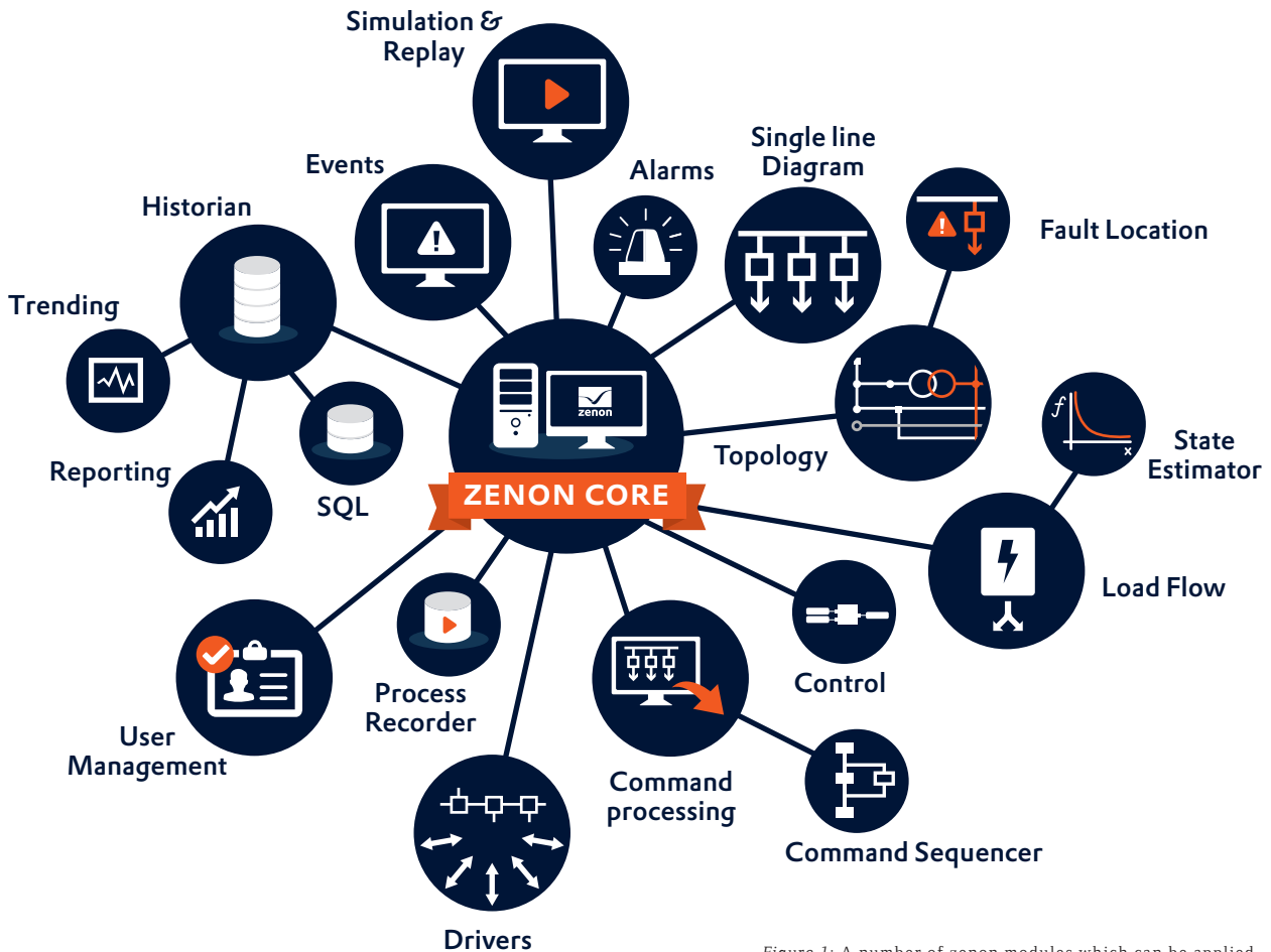
Figure 1: A number of zenon modules which can be applied to control and monitor a distribution network system for smaller to mid-sized municipal utilities.
