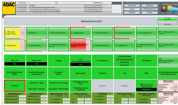
Figure 1: Status of all areas at a glance. Faults and messages are color-coded.
