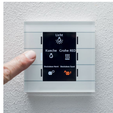
A modern KNX Push Button can operate up to 24 actions. Robert Merz carries out primary tasks in zenon, which the KNX telegrams then process.
