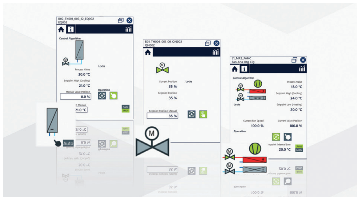
Figure 1: The image shows three smart objects, an air cooler, a valve, and a heater, each displayed with their respective process-related information on faceplates (pop-ups). These faceplates highlight key operational data and parameters, demonstrating how smart objects provide real-time visibility and control within the system.
