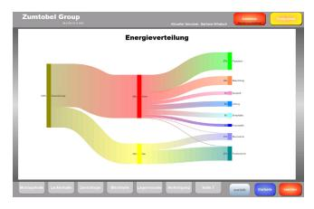
The Sankey Diagram clearly displays the energy consumption of Zumtobel's painting hall.
