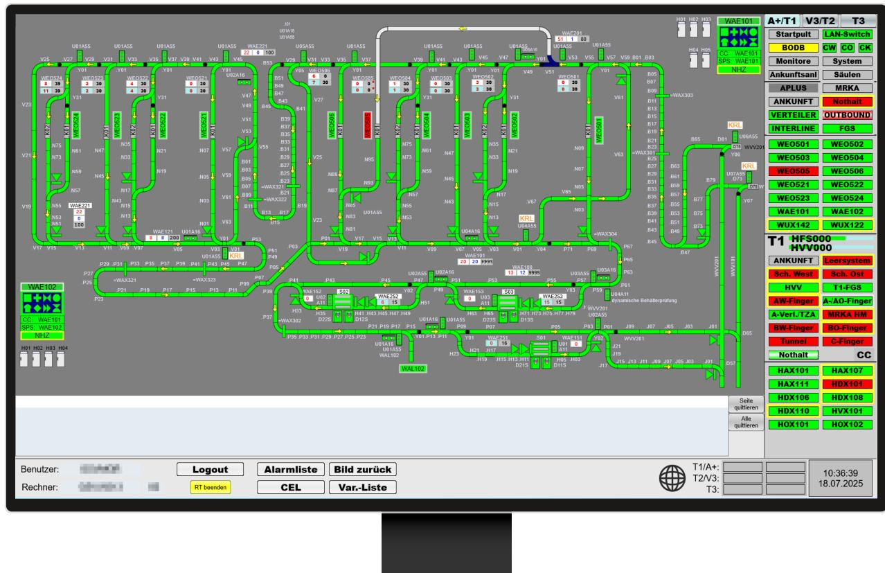
The first gate in Terminal 1 visualized with zenon, including incoming and outgoing conveyor lines and collection points.
