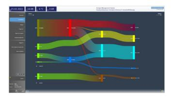
The Sankey diagram in the Microgrid EMS clearly visualizes all energy flows from producers to consumers.
