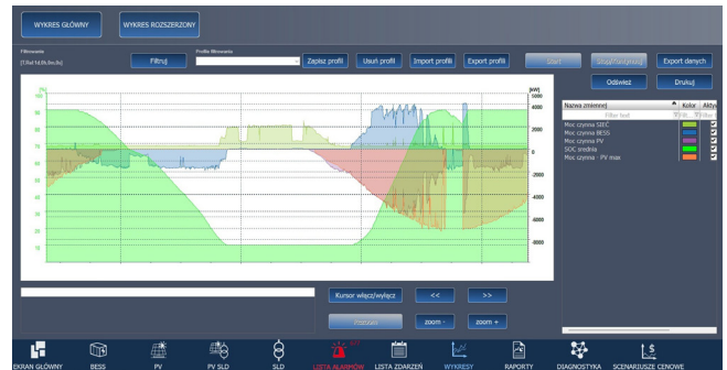
Chart showing the operation of the PV system and BESS provides a comparison of the active power of the sources and the state of charge of the batteries on a daily basis.
