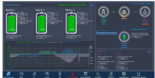
A screenshot of the EMS operator desktop shows the operational status of the storage facility and the PV farm.
