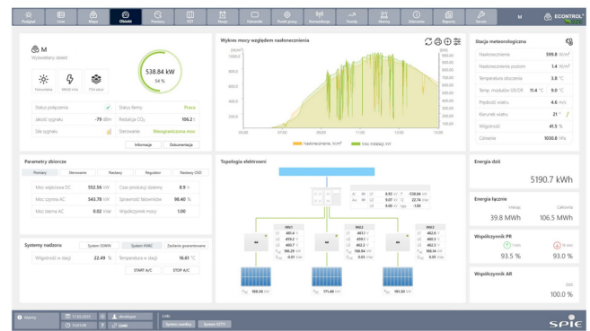
Fig. 2. Main screen of a PV farm
