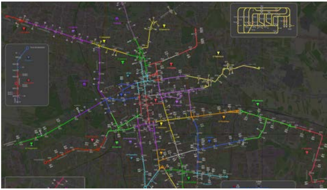
View of over 30 tram substations in Łódź and nearby towns with integrated automatic line coloring and visual alarms.
