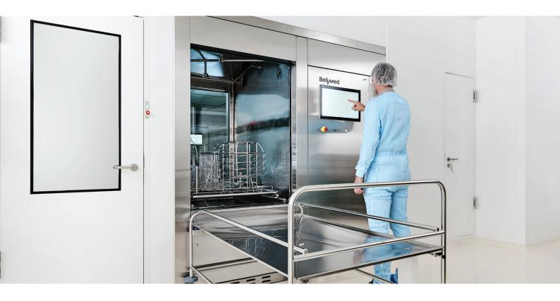
Sterility is critical in pharmaceutical manufacturing: machine parts, containers, and packaging have to be sterilized prior to every use. This is usually done under pressure with steam in sterilizers, which are used in the pharmaceutical industry for medications and their initial packaging. To meet regulatory requirements, sterilizers must eliminate viable microorganisms.
